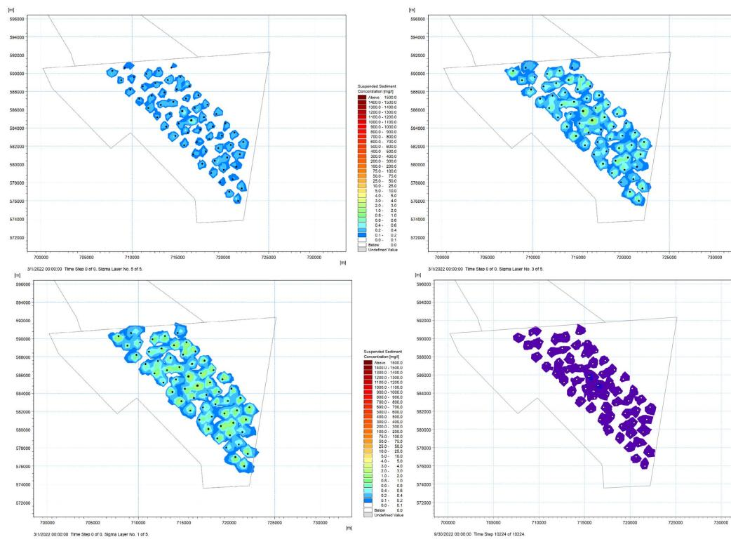
Figure 8-24 Maximum Predicted Suspended Sediment Concentrations Released in the Surface Layer (top left), Middle Layer (top right), and Bottom Layer (bottom left) due to Foundation Installation by Drilling. Total Sediment Deposition Thickness is shown bottom right
