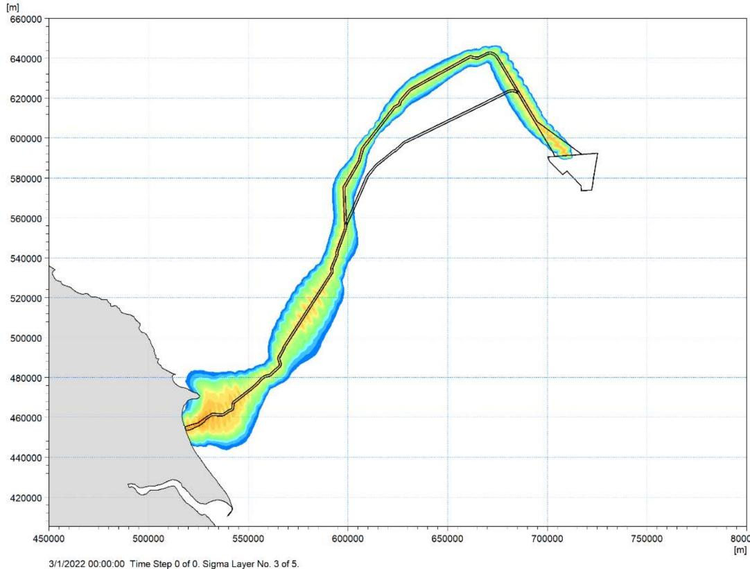
Figure 8-34 Maximum Predicted Suspended Sediment Concentrations Released in the Middle Layer due to Trenching for Offshore Export Cable Option 1 route
