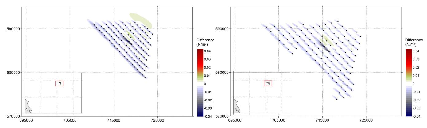
Figure 8-43 Difference in Maximum Bed Shear Stress over 30 days between Baseline and Windfarm using Turbine Layout B (left) and Turbine Layout C (right)
