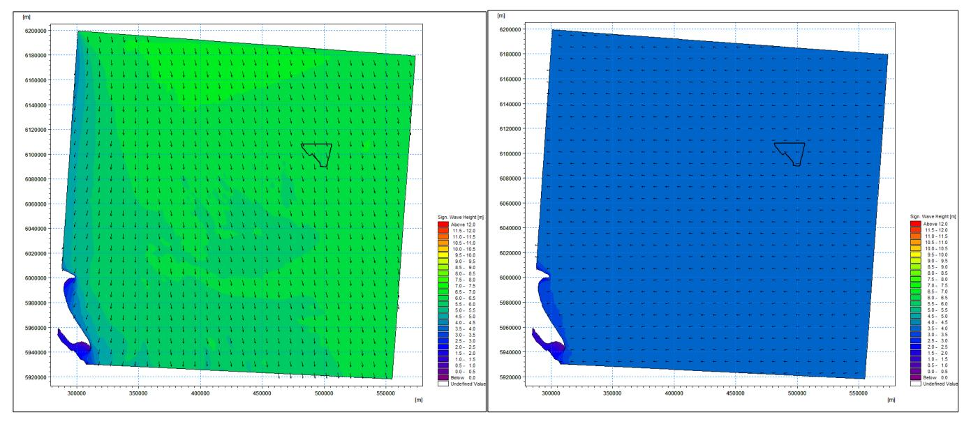
*Figure 8-10 Predicted Baseline Significant Wave Height for 1 in 1 year Return Period Waves Approaching from the North (left) and East (right)*
