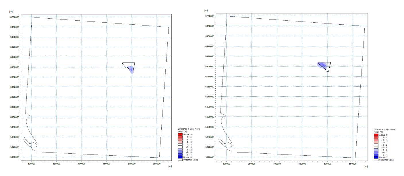
Figure 8-42 Percentage Difference in Significant Wave Height between Baseline and Windfarm Turbine Layout C for Waves Approaching from a northerly direction during a 50th Percentile Return Period event (left) and Waves approaching from the East during a 50th Percentile Return Period Event (right)
