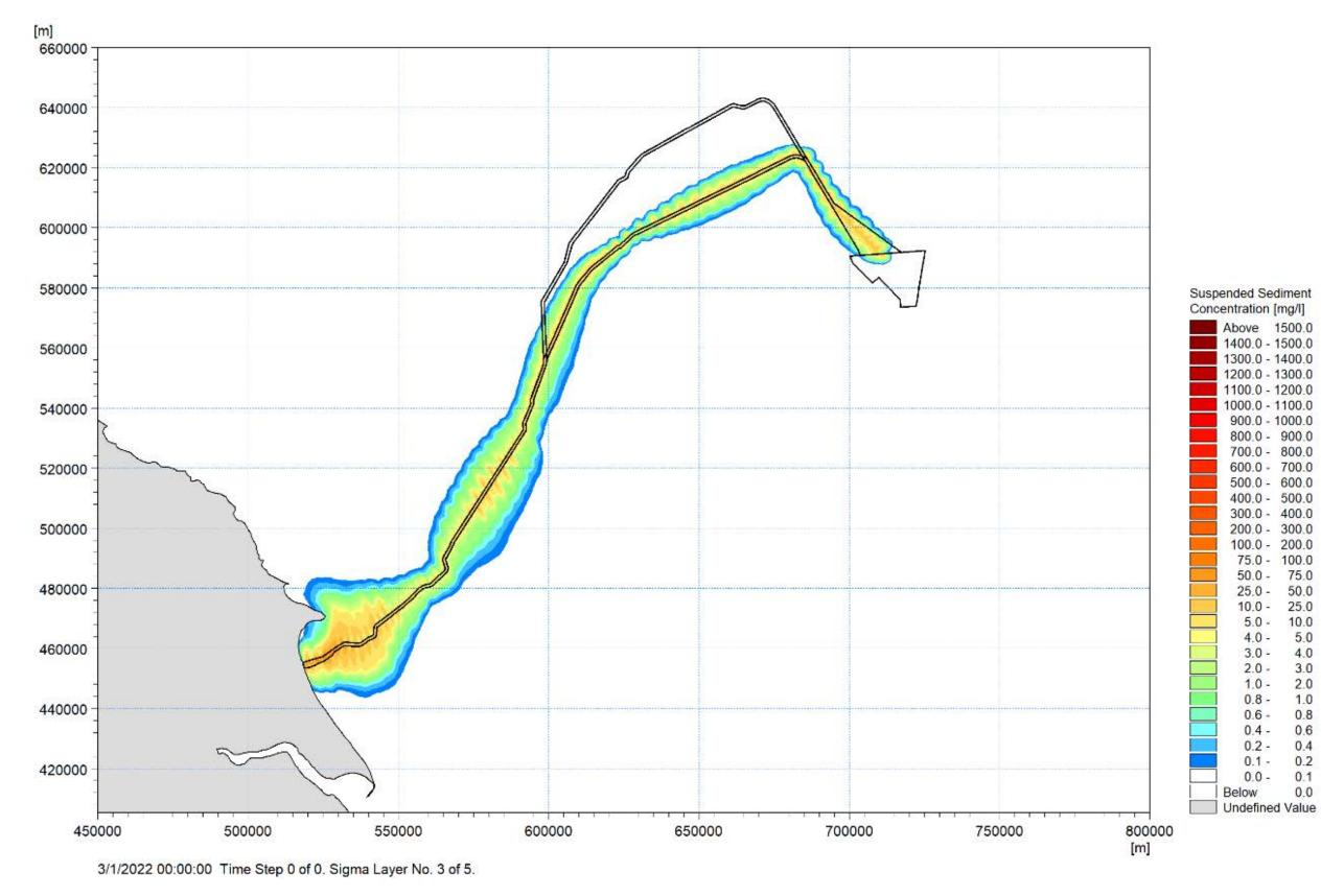
Figure 8-38 Maximum Predicted Suspended Sediment Concentrations Released in the Middle Layer due to Trenching for Offshore Export Cable Option 2 route
