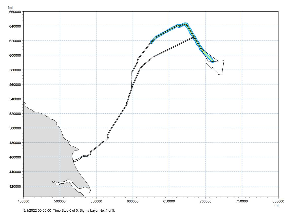
Figure 8-27 Maximum Predicted Suspended Sediment Concentrations Released in the Bottom Layer due to Sand Wave Levelling for Offshore Export Cable Option 1 Route
