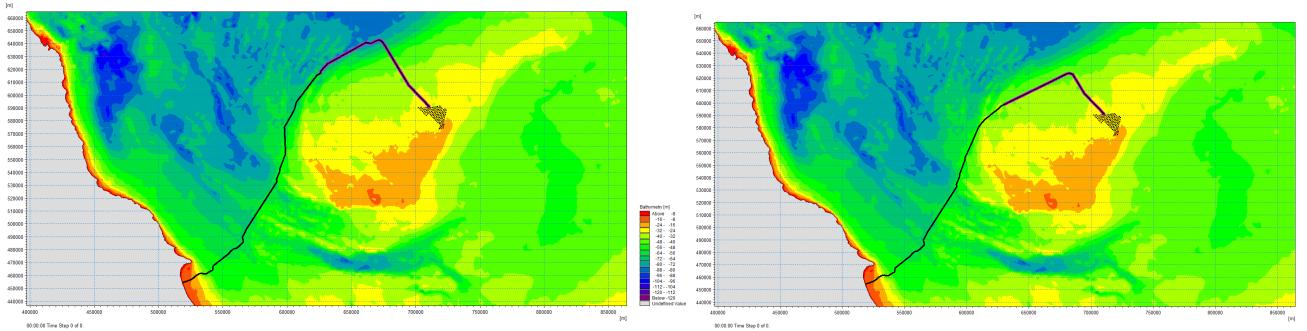
Figure 8-3 Modelled Offshore Export Cable routes. Option 1 (left) and Option 2 (right). The thicker (purple) line shows where sand wave levelling would be required
