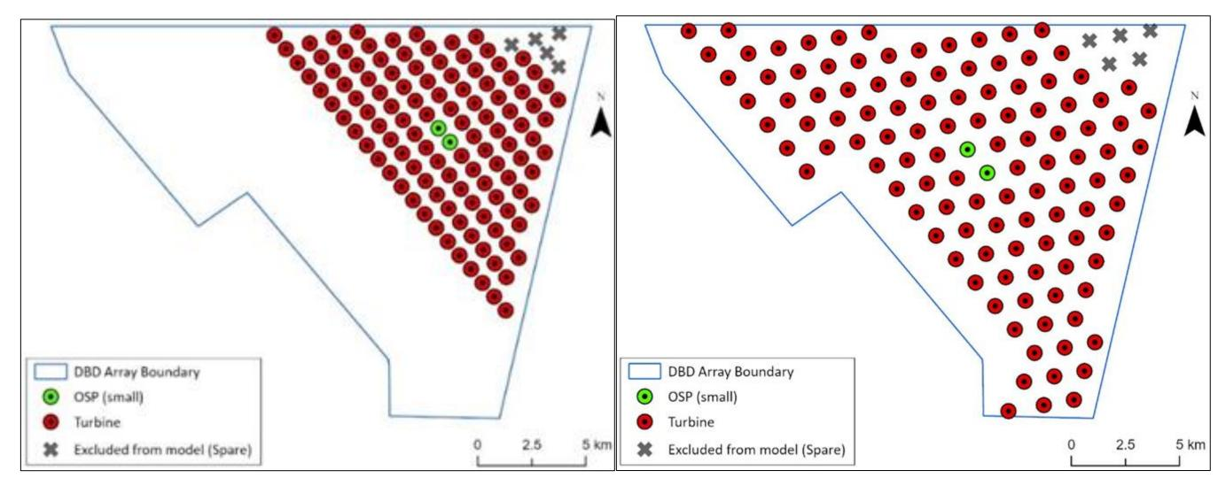
Figure 8-2 Worst-case Scenarios for the Project for tidal currents (Layout B) (left) and for waves and sediment dispersion Layout C) (right)
