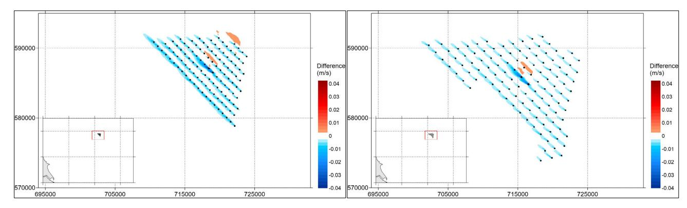
Figure 8-41 Difference in Maximum Current Speed over 30 days between Baseline and Windfarm using Turbine Layout B (left) and Turbine Layout C (right)
