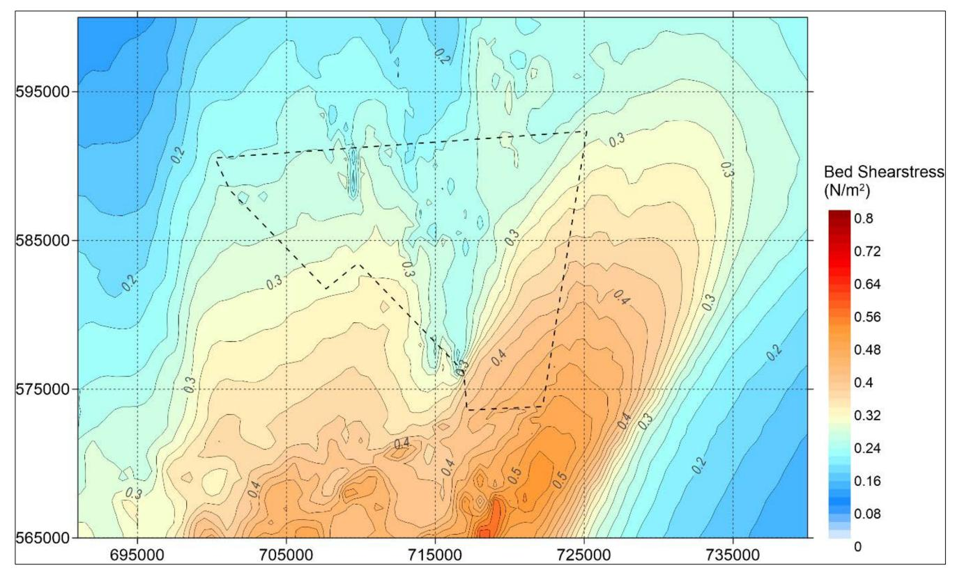
*Figure 8-13 Predicted maximum bed shear stress over 30 days*
