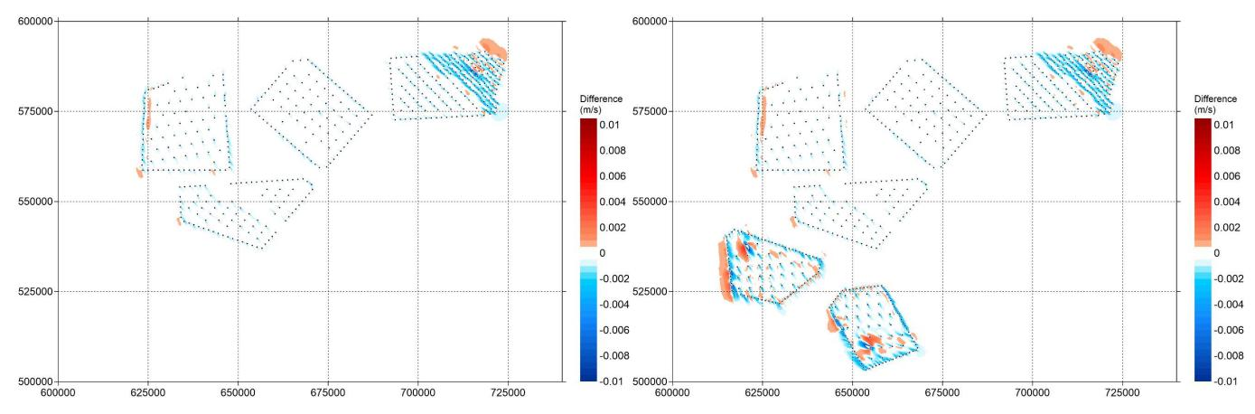
Figure 8-44 Cumulative difference in Maximum Current Speed over 30 days between Baseline and Option 1 (left) and Option 2 (right) (Turbine Layout C)
