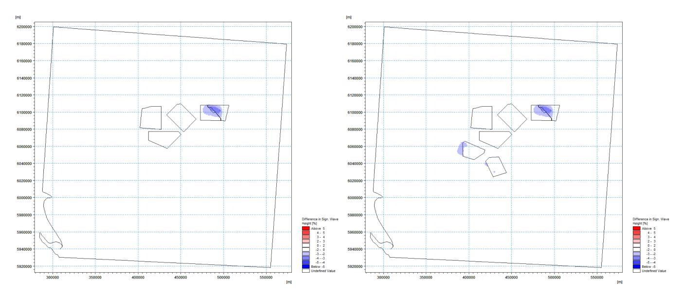
Figure 8-46 Cumulative Percentage difference in Significant Wave Height between Baseline and Option 1 (left) and Option 2 (right) (Turbine Layout C) for Waves Approaching from an easterly direction during a 50th Percentile Return Period Event
