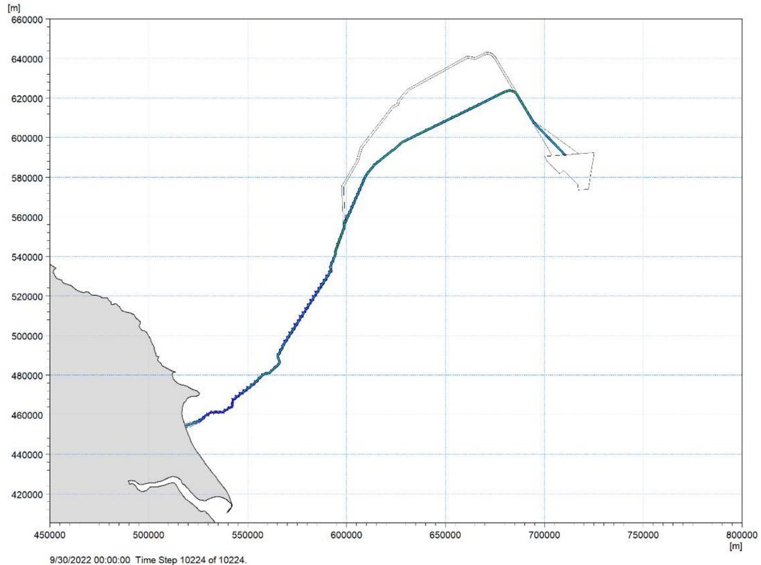
Figure 8-40 Total Sediment Deposition Thickness due to Trenching for Offshore Export Cable Option 2 route
