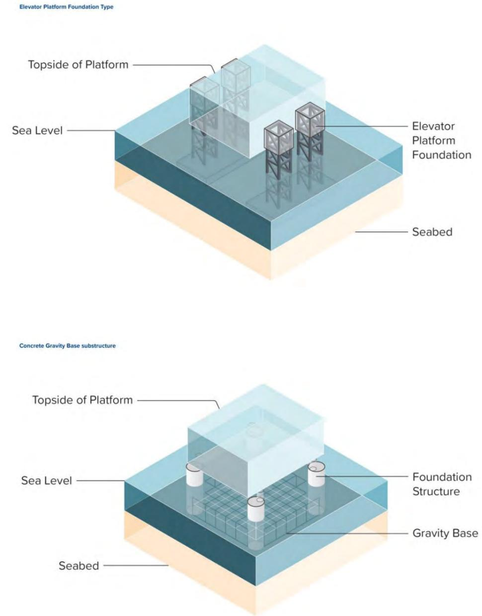
Plate 3-3 Potential Offshore Platform Foundation Types
