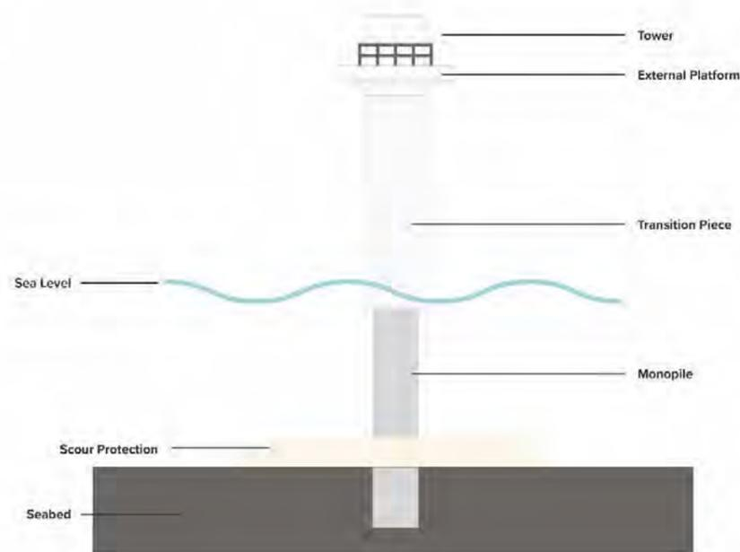
Plate 3-2 Potential Wind Turbine Foundation Types
