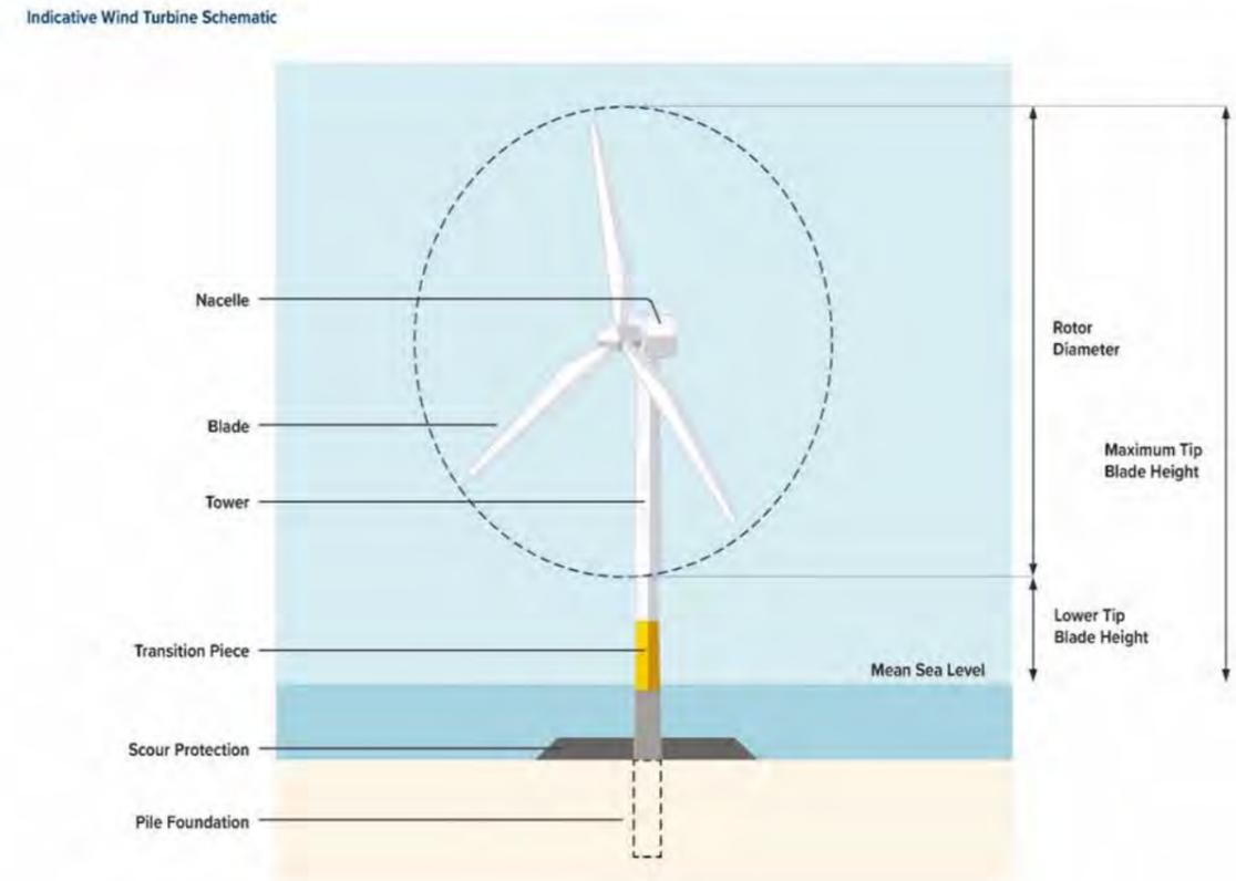
Plate 3-1 Indicative Wind Turbine Schematic
